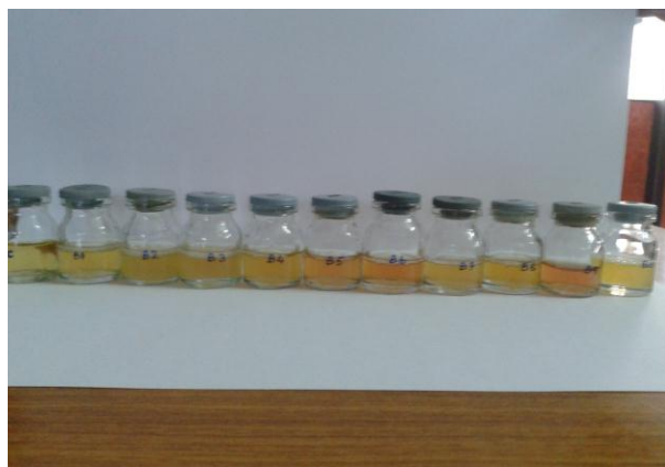
Fig 6: Detection of lead ion by GSH-AgNPs in blood samples
